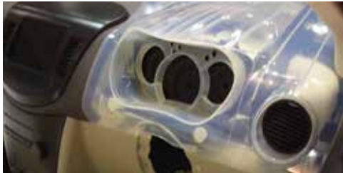
Various Accura materials for form and fit tests of a dashboard
