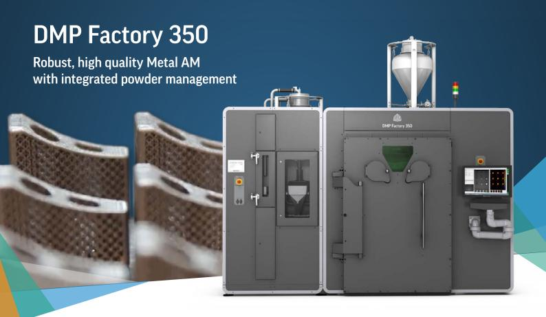
High throughput, high repeatability metal 3D printer that generates precision quality parts from the most challenging alloys with high quality material management for maximum powder usage. Integrated metal 3D printing solution with DMP production metal printer, 3DXpert™ software, thoroughly qualified LaserForm® materials and expert application support. For companies that are scaling their metal AM production and require closed powder handling.
